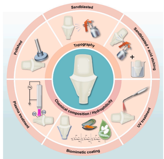
Fig. 1. Surface modification of zirconia abutment.
